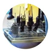
Ergonomics - non-gloved, gloved, gloved & blindfolded Noise Cancellation - fan, chainsaw, pump panel, SCBA, PASS alarm Immersion - 3' of water in a barrel for 30 minutes Humidity - in a dishwasher for 1.5 hours on hot cycle Temperature Extremes - oven drawer to freezer & back (10 minutes in each for 3 cycles) Drop - 6' & 10' horizontal & vertical onto a concrete floor Vibration - bubble wrapped in a paper collator for 5 minutes
